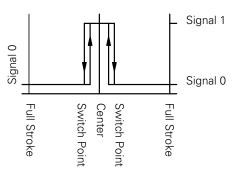
Signal 0 = Voltage at pin 2/4 < 1.8VSignal 1 = Voltage at pin 2/4 > (Vs - 2.5V)
