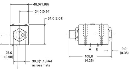
Pilot/drain connection  $B-G1/8\ thread$ S -SAE straight thread (7/16"- 20 UNF)
