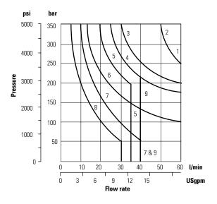
**Graph 2** AC solenoid valves operating at 60 Hz
