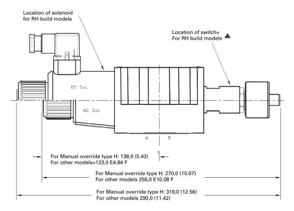
▲ For LH models ("L" in model code location 4) solenoid and switch locations are reversed ∆ Wiring: See warning note on page 118
