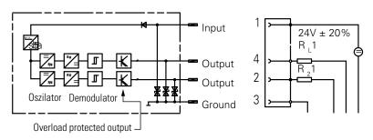
$R_1$ 1,  $R_1$ 2 = e.g. Coil Resistance of the switch relay >/ = 60 OHMS
