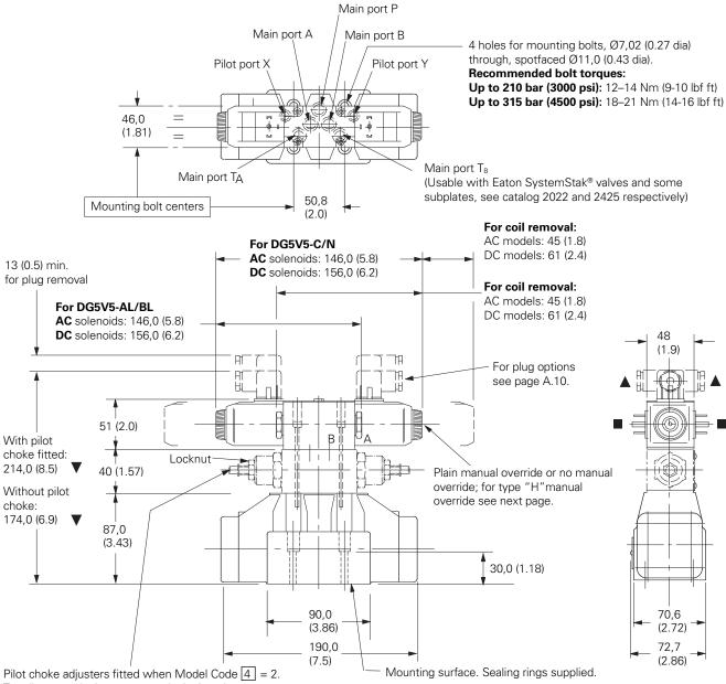
Pilot choke adjusters fitted when Model Code [4] = To adjust, turn locknut counter-clockwise, then turn screw clockwise to slow down rate of spool travel, or counter-clockwise to increase the rate.
