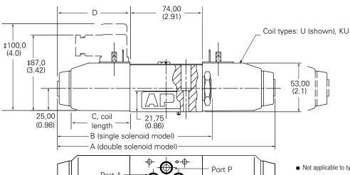
Alternative plug positions by loosening knurled nut, turning coil, and re-tightening.
