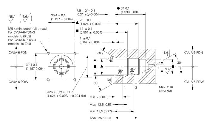
◆ Tool kit 459285 for machining the Ø17 mm, Ø18 mm and Ø19 mm bores (and when required, the Ø26 mm bore) can be ordered if required. The kit comprises a stepped drill and a stepped reamer.
