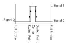
Signal 0 = Voltage at pin 2/4 < 1.8VSignal 1 = Voltage at pin 2/4 > (Vs - 2.5V)
