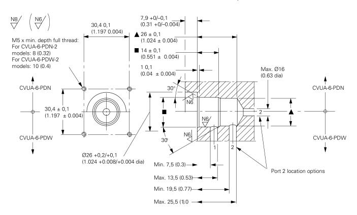
◆ Tool kit 638692 for machining the Ø18 mm and Ø19 mm bores (and when required, the Ø26 mm bore) can be ordered if required. The kit comprises a stepped drill and a stepped reamer.
