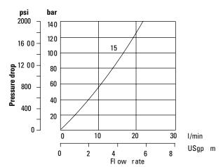
▼ Curve for spool type 6: not recommended for flows in excess of 60 l/min (15.8 USgpm).
