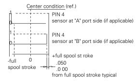
1= voltage at pin 4 (Vs – 2.2V) min. 0= voltage at pin 4 0.5V min.
