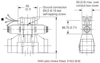
With pilot choke fitted: 218,0 (8.6) Without pilot choke: 178,0 (7.0)
