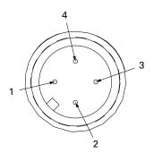
**Pin 1** is only used on the Z option for 24 VDC power to the valve.
